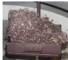
U product collected during advanced refiner tests
